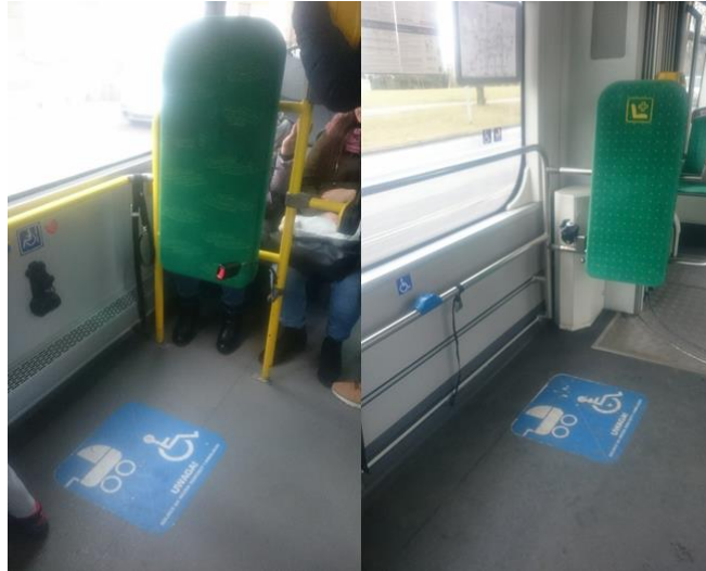
Fig. 8. Places marked for disabled persons on the bus (left) and low-floor tram (right). Push buttons for persons needing support during exit, safety belts as well as cushions are seen on the photos. Own elaboration
