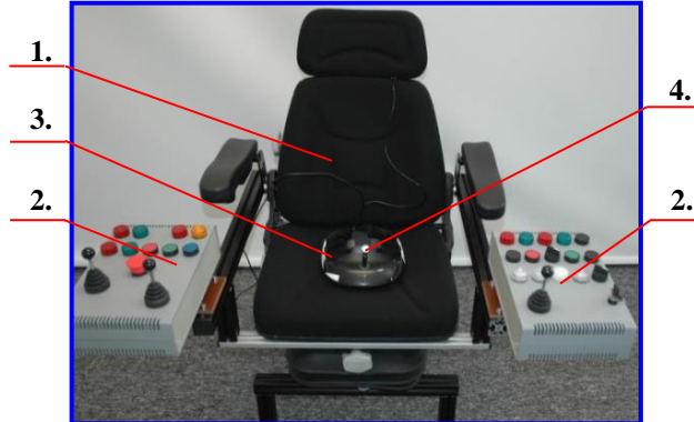
Fig. 1. View of the overhead crane simulator: 1- seat of the simulator, 2- real panels to control the virtual overhead crane functioning in the simulator, 3- infohelmet, 4- motion sensor of the tracking system.
