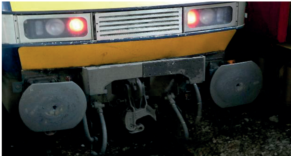
Fig. 11. Hybrid coupler combining a screw coupler and an AAR coupler (HandWiki, 2025)
