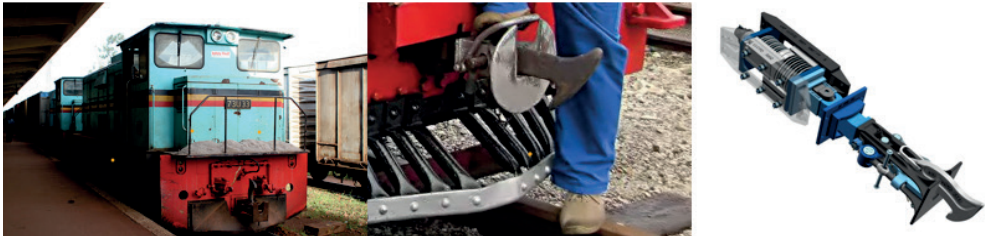
Fig. 3. Bell and hook coupler (Wikipedia, 2025a)
