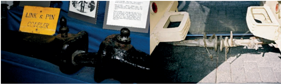
Fig. 2. Link and Pin Coupler (Wikipedia, 2025a)
