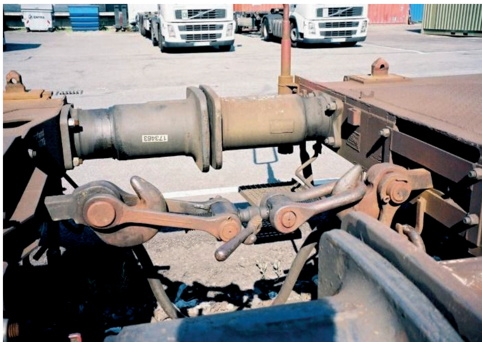
Fig. 7. Draft and Buffing Gear with Screw Coupler (Wikipedia, 2025b)
